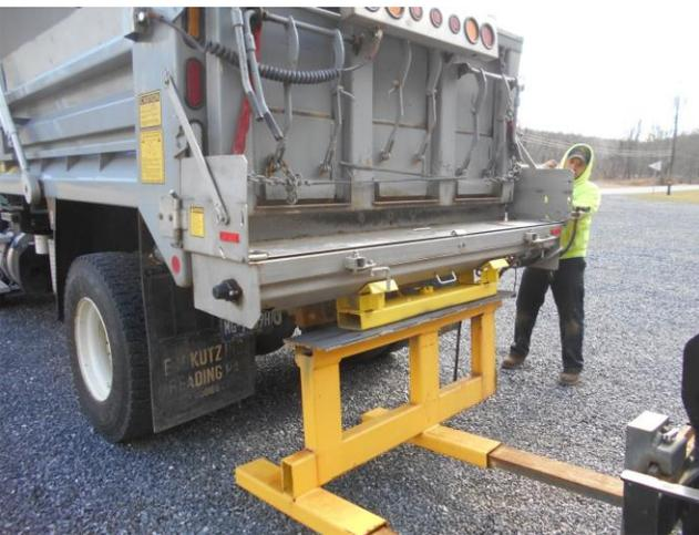
block wall and a sliding mechanism so that a backhoe with forks can lift the spreader off the wall and onto a truck for installation. The system allows the spreader to be installed without having to put it down and lift it again.
