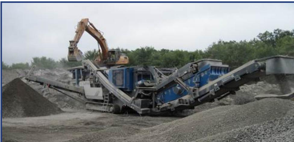
Crushed concrete pavement is processed and used in new pavement applications. Pennsylvania currently limits the use of CCA to unbound applications in pavement structure.
