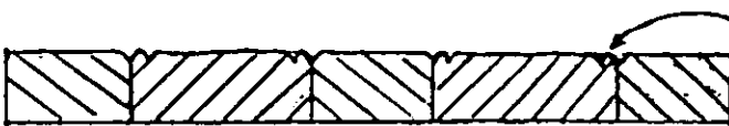
detail of door showing stiles + rails with the beads on the panels
