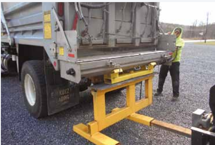
This system of heavy-duty shelving with a sliding mechanism makes it easier to store a tailgate spreader and install it onto a truck without having to put it down and lift it again. South Manheim Township, Schuylkill County, 2017 Runner-up
