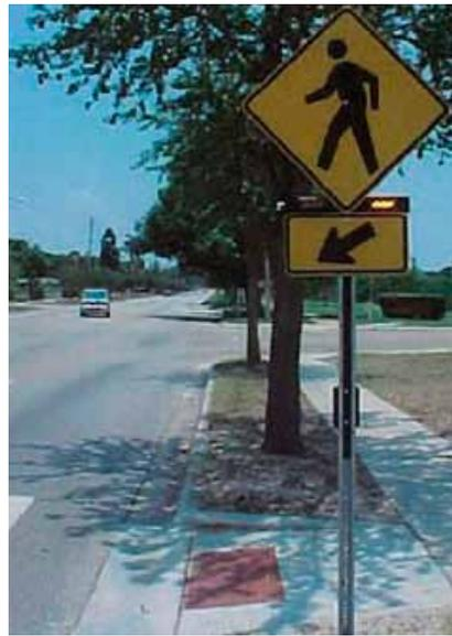
Rectangular rapid flashing beacons have been approved once again by FHWA now that patent issues with the device have been resolved.
