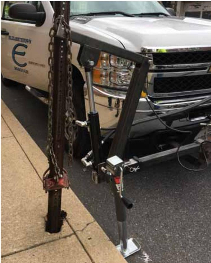
Bath spent about \$150 in materials to adapt a 1,000-pound crane that can be mounted on the rear of its street sweeper and used to hoist a storm sewer grate. The crane, which only requires one person in one vehicle to operate, makes it easier and safer to access storm sewer basins for cleaning.
